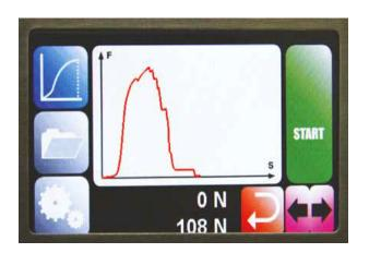
The straightforward design of the user interface with a **colour touch-screen** and **intuitive menu navigation** simplifies operation and enables reproducible test results. The **force-time characteristic** is displayed as a **curve on the screen**. The measured values can be saved to a SD card and retrieved later. This also enables statistical analyses to be carried out on the device.
